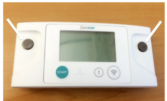
Figure 1: The Zenicor-ECG device with the dimensions of 145 × 65 × 25 mm and a weight of 135 g. To record a 1-lead ECG the thumbs must be placed on the electrodes (arrows) for 30 seconds. The ECG strip is sent via 2G mobile-connection to a web-based service (Zenicor-ECG Doctor System).
